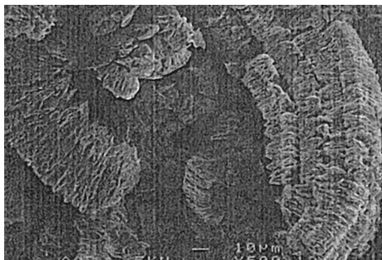
Fig. 1. SEM micrograph of graphite A.1.1 after one cycle in PC/EC/3DMC \text{LiPF}_6 1 M.
